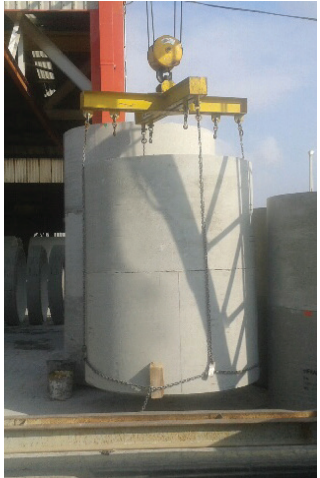
Photo depicting an alternative method of correct lifting gear.
