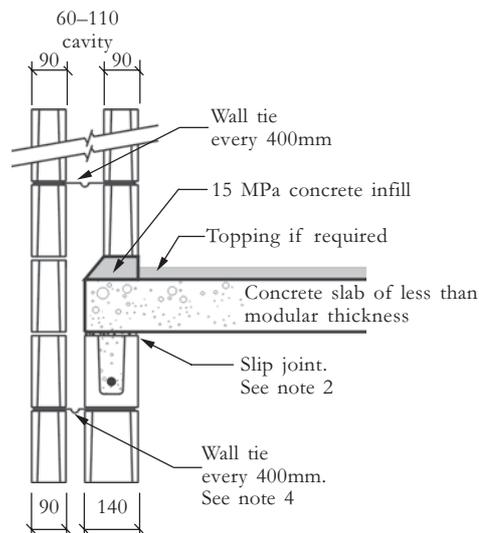
**WALL: INNER LEAF -STRUCTURAL BELOW SLAB
