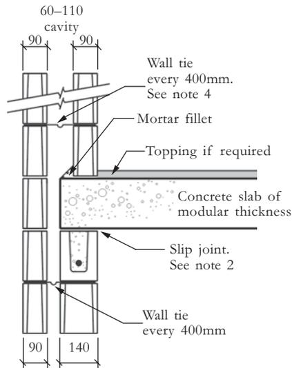
**WALL: INNER LEAF -STRUCTURAL BELOW SLAB
