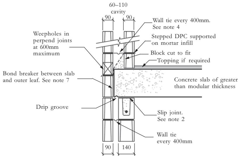
**WALL: INNER LEAF -STRUCTURAL BELOW SLAB
