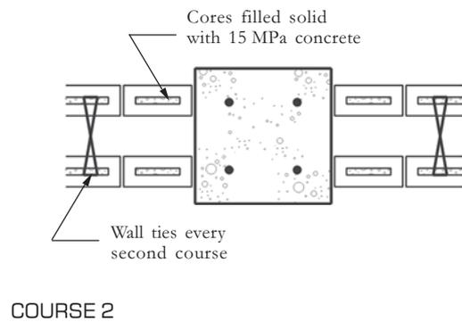
**WALL LATERALLY SUPPORTED BY CONCRETE COLUMN, PERMITTING LONGITUDINAL MOVEMENT IN WALL**
