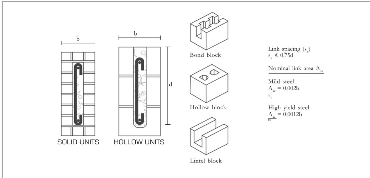
Where compression steel is used in beams, links should be provided as for columns. Column links are required when the area of steel exceeds 0,25% of the gross area of the column and the design load exceeds 25% of the resistance capacity of the column. In such circumstances, links should be provided as follows:
