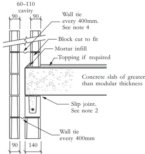
**WALL: INNER LEAF -STRUCTURAL BELOW SLAB
