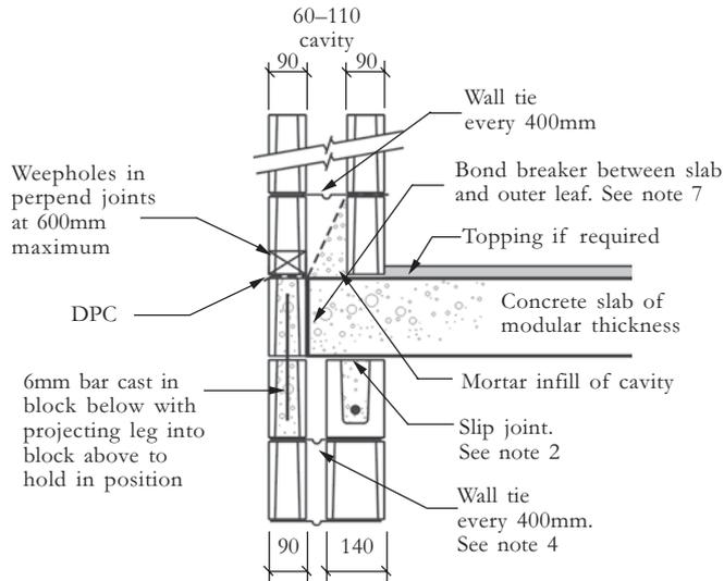
**WALL: INNER LEAF -STRUCTURAL BELOW SLAB
