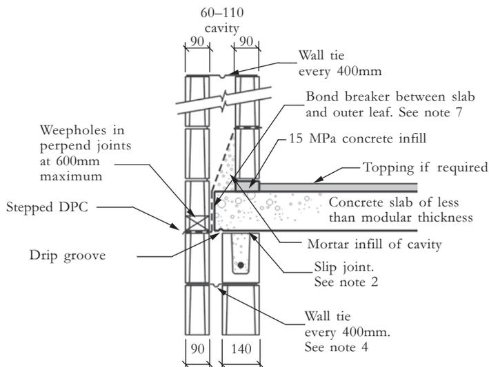
**WALL: INNER LEAF -STRUCTURAL BELOW SLAB
