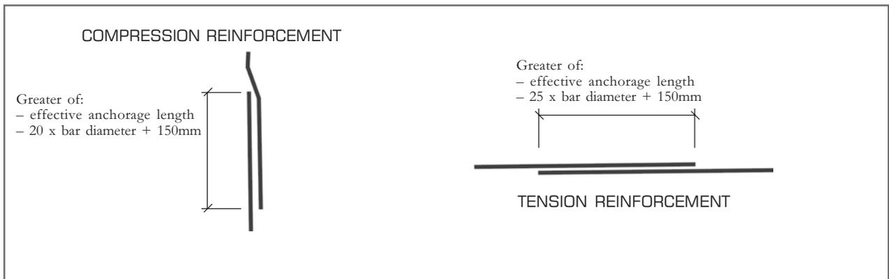
Generally, laps should be located away from areas of high stress and should be staggered. Account of the construction sequence, buildability, stress considerations, congestion of reinforcement etc., should be taken in the location of laps and joints.
