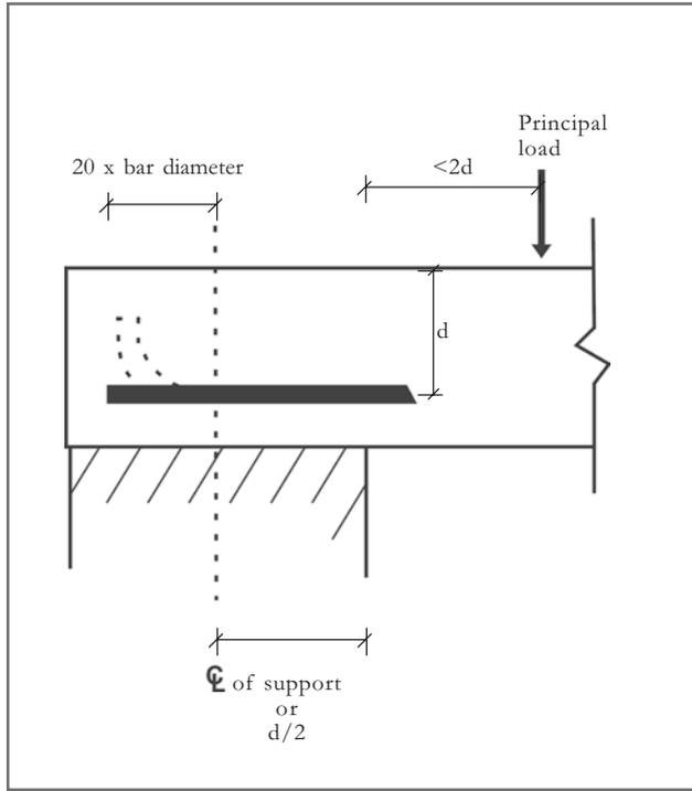
Reinforcing bars which are subjected to bending and terminate other than at an end support, should continue for a distance beyond the point at which they are no longer required, equal to the greater of the effective depth of the member or 12 times the bar size, provided, however, that one or more of the following is satisfied:
