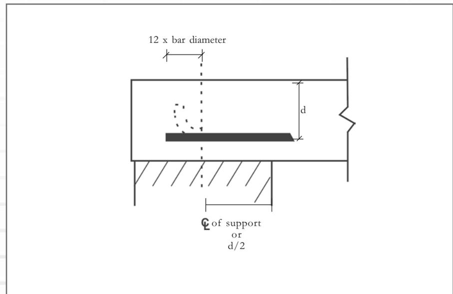
However, should the distance between the face of the support and the edge of the nearest principal load be less than twice the effective depth, reinforcement should be curtailed as follows:
