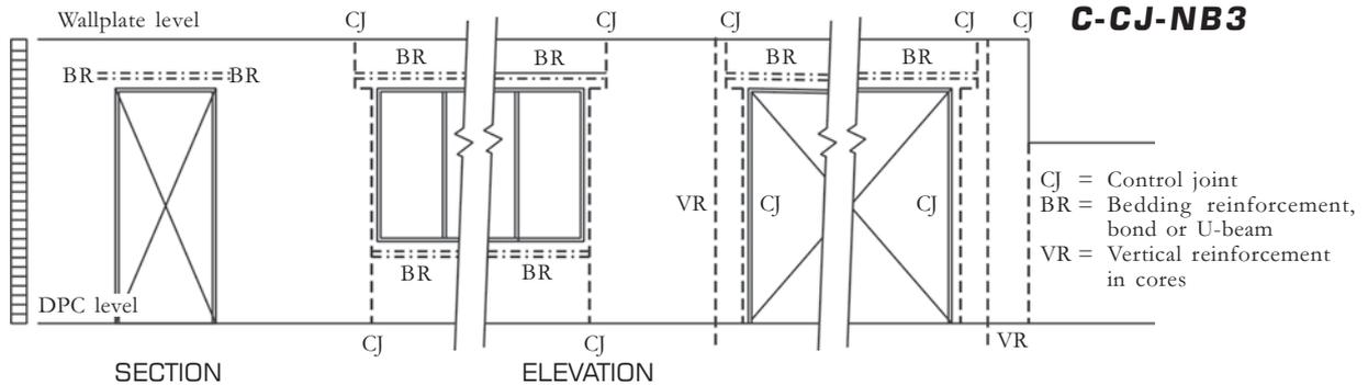
**ELEVATION OF WALL SHOWING CONTROL JOINT POSITIONS AT EDGE OF OPENINGS, HORIZONTAL & VERTICAL REINFORCEMENT**
