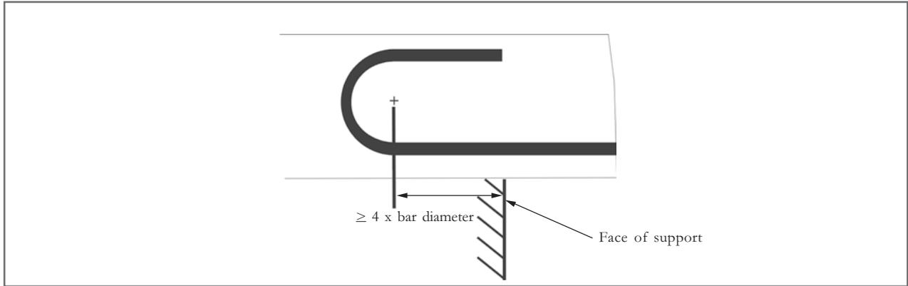
Joints in reinforcement may be achieved by means of mechanical couplers or simply by lapping reinforcing bars of follows:
