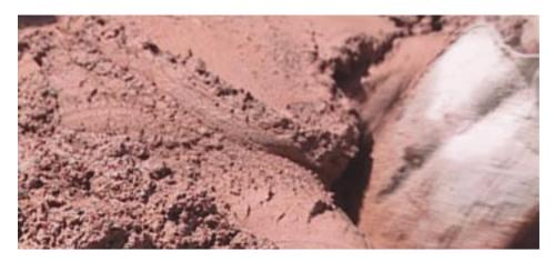
The mortar must be thoroughly mixed and suitably tinted to the colour of the tiles.
