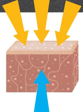
Efflorescence emerged from pores within a magnified area of a concrete paver. The calcium has been carried to the surface by water.
