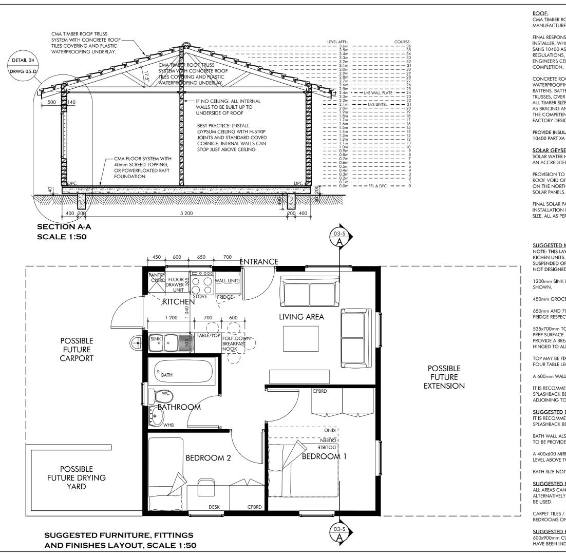
CMA TIMBER ROOF TRUSS SYSTEM, BY AN APPROVED MANUFACTURER AND INSTALLER.
