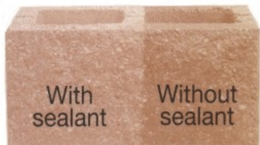
The effect of sealant on wetted concrete masonry
