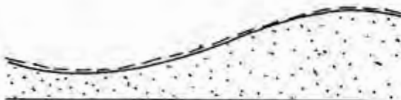
USE OF SHORT SCREEDING RAILS TO GAUGE THE CURVATURE
